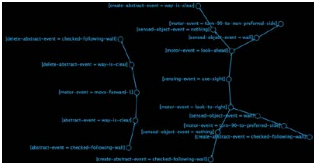
Figure 6.5 Screenshot of the Wall Following Events model defining the modified wall following behaviour.
